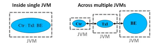
There is always exactly one Controller component and at least one Backend. Each Backend has one or more dedicated Transaction Injector(s) mapped to it. This logical mapping is called a "*Group*". The topology for a *Group* can be defined using command line options in the run script.
